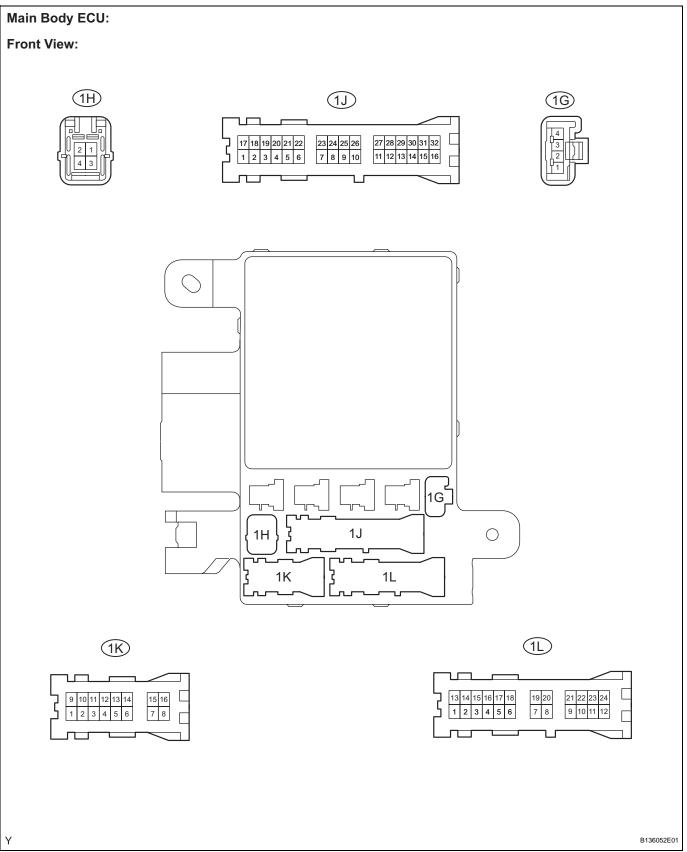
(a) Disconnect the 1A, 1B, 1E, and 1H main body ECU (driver side J/B) connectors.
